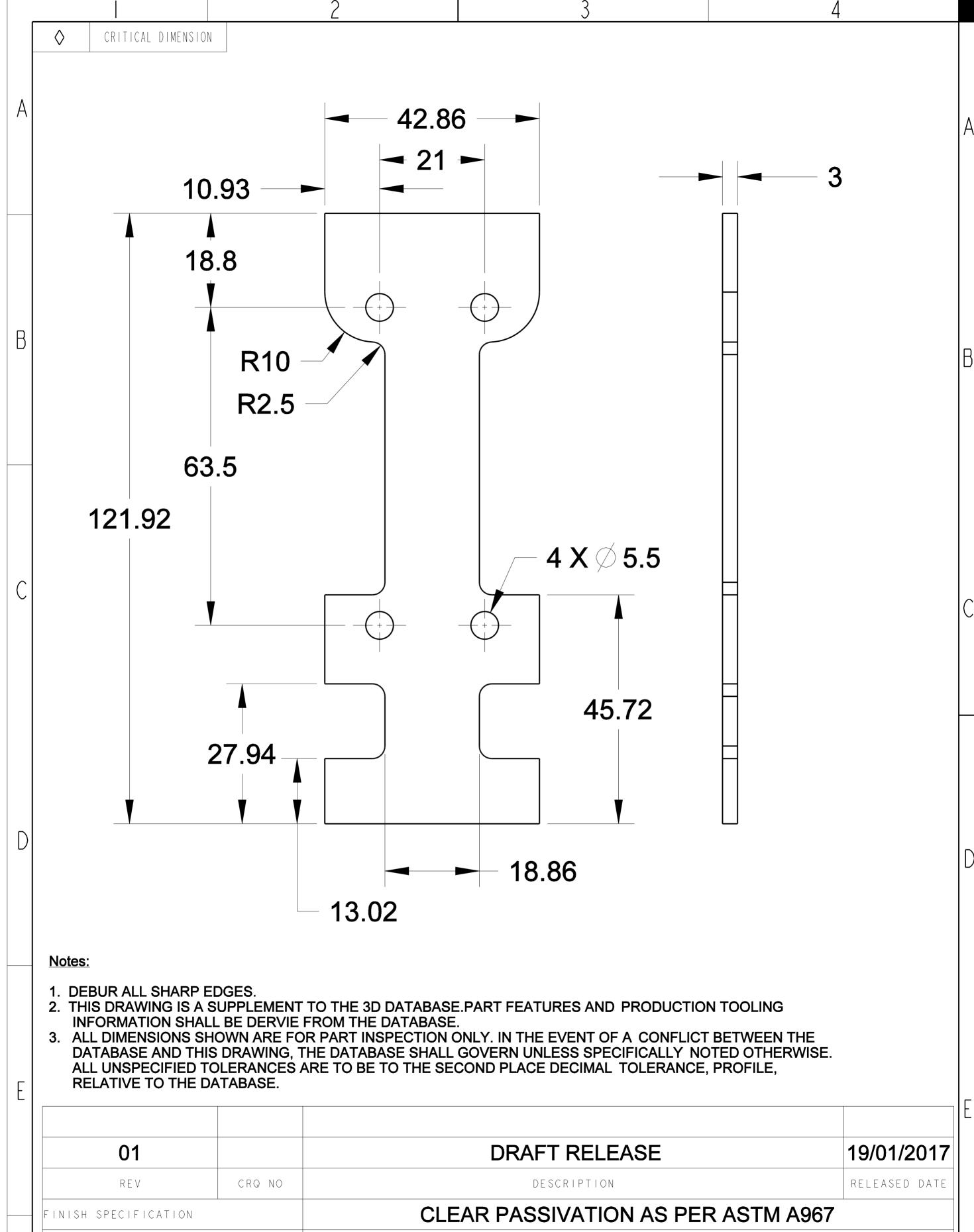
SS 316 (SHEET METAL) MATERIAL SPECIIFCATION UNLESS OTHERWISE SPECIFIED LINEAR TOL=1SO 2768-M 0.5 - 3 :+/-0.10 DOCUMENT CODE PART DRAWING 3-6 :+/-0.15 6-30 30-120 : +/-0.20 : +/-0.30 **OpenCellular** THIRD ANGLE UNIT SCALE **PART NAME** Mechanical, Plate, Rear, weldment 1.000 SHEET SIZE **PART NO** 227-001334 SHEET 1/1 A 4
